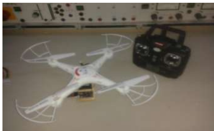
Fig. 12 Installation of the instrumentation on the quadrotor
